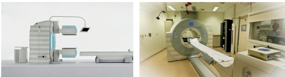
Figure 1. Left image: gamma camera with SPECT-CT possibility (Siemens Symbia T). Right: PET-CT camera (Siemens Biograph mCT 64-slice).
